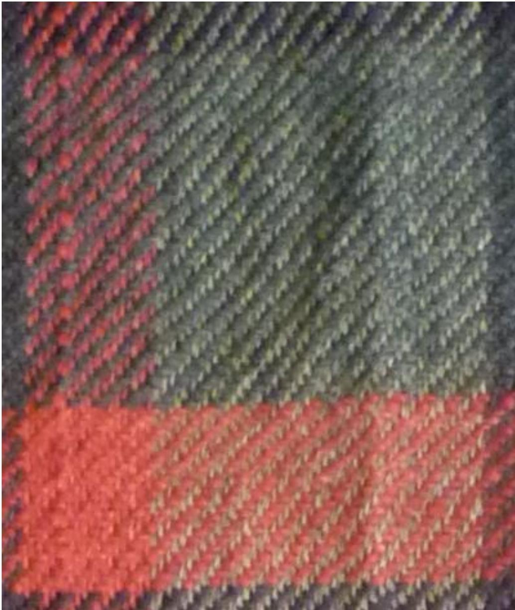
Plate. 4 Detail showing the difference in the warp (light) and weft (dark) green yarn shades.
